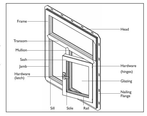
Figure I Components of a window
