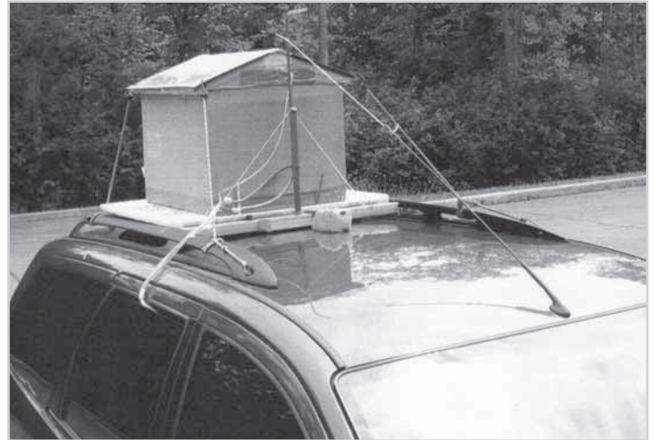
Figure 1 Model House Being Mounted for Airstream Testing Pitot tube is visible at top of photo, above and forward of gable roof peak. The house stance can be adjusted to any angle "to the wind." The twin manometers are mounted inside off the sun visor. Observer: Peter Russell, PEng
