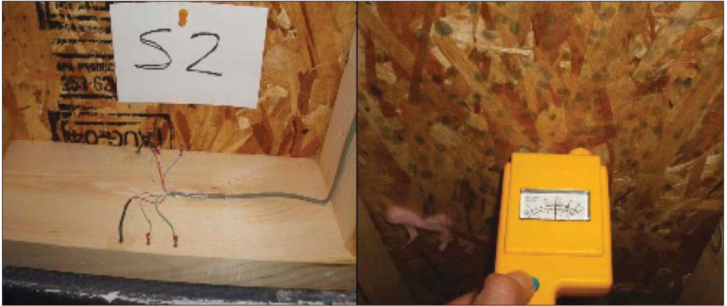
Figure 1 Stain-free south-facing no-polyethylene (left) and mold spots on north-facing no-polyethylene wall
