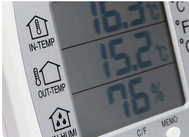
A hygrometer is an instrument used for measuring the moisture content in the atmosphere.
